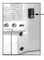
Insert the plug on the end of the supplied power cord into the AC power jack on the back of the radio.
